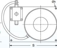
A complete Dynemech DLPM system consists of three master pneumatic isolators for 3 point precision leveling. Each pneumatic damping isolator consists of a leveling valve which is the load sensing and height controlling element. Systems are supplied with automatic height control valves, tubing and all other pneumatic accessories necessary for complete system installation. Dynemech DLPM Mounts have minimal setting time.
