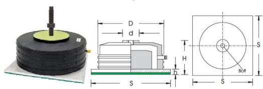
Dynemech Rubber Air Springs provide highly effective insulation of machines against low frequency vibration/impact. The element offers a vertical natural frequencies between 2.5 to 6.0 Hz\*. The component has vertical to horizontal stiffness ratio of approx imately one. Suited for both active and passive vibration control.
