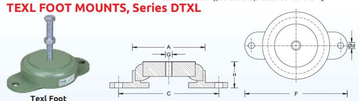
Low cost solution for Shock Absorption and Vibration control. Rugged CI body mount provide option for low height machinery installation option. Simple, ready to install configuration with top cup and bottom base plate bolting options. Provides stability, smoother operation and reduced maintenance in machinery. High efficiency, stable fixed support, long service life of mounts ensures greater productivity of machinery.
