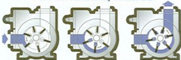
FIGURE 1. How Blackmer's sliding vane action works
