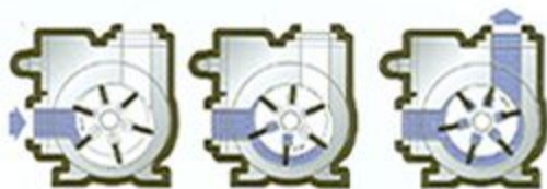
How Blackmer's sliding vane action works
