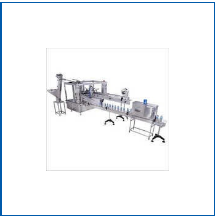
BOTTLE RINSING FILLING AND CAPPING MACHINE
