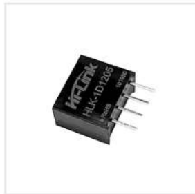
HLK 1D1205 ENERGY PROVIDE MODULE
