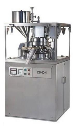
• It is square GMP model Single Rotary Tablet Press. Operator friendly design, provided with electronic digital tablet cum RPM counter. Reverse direction motion protection is also provided for safety purpose.
