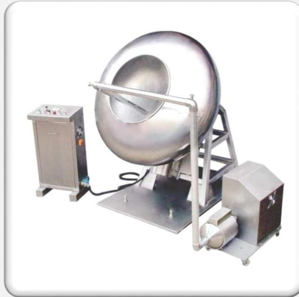
Coating Machine is available with 12", 24", 30", 36", 42", 48", 60" or 72", size SS Pan. Coating Machine is totally enclosed with MS Cladding with standard Gear Box, Motor, Hot Air Blowing arrangement. Machine is designed with MS fabricated structure and all arrangement – except electric control, air filter and SS Pan are inside the enclosure, which makes simple cleanable outside covering.
