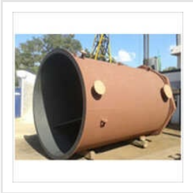
Rubber Lined MS Tank
