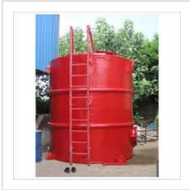
FRP Lining Of MS Tank
