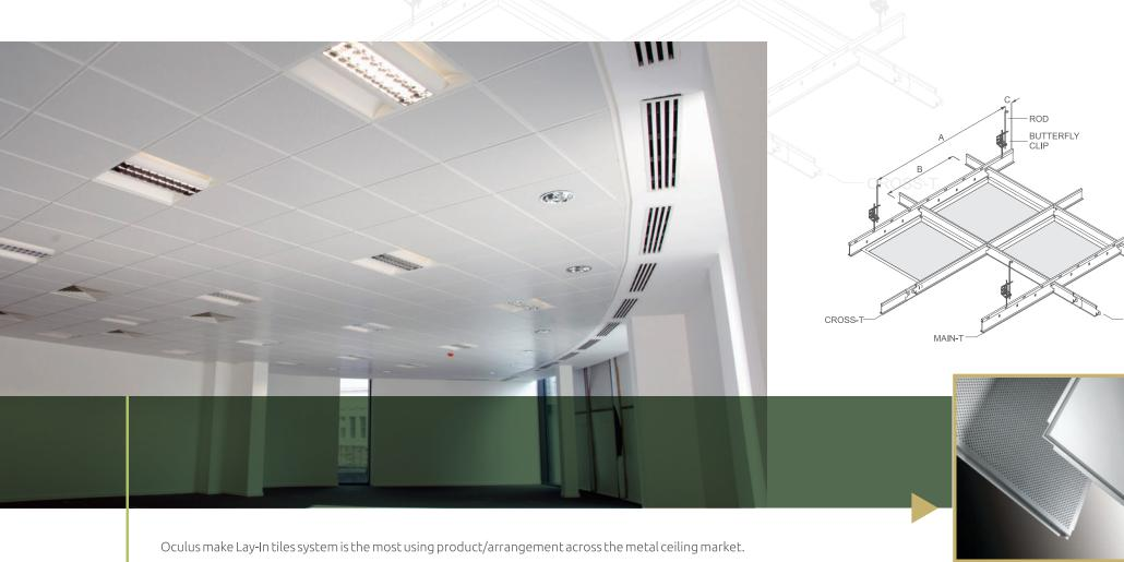
The visible 24mm, 15mm plain & 15mm silhouette T- grid make it more elegant and provoke customer to use, Tiles being stove enamelled Aluminium/ Galvanized are fully recyclable with the use of small amount of energy, Lay-In tiles are available in different thickness & sizes 575\*575, 585\*585, the system creates a modular arrangement of 600\*600. Lay-In tiles system is simple to install
