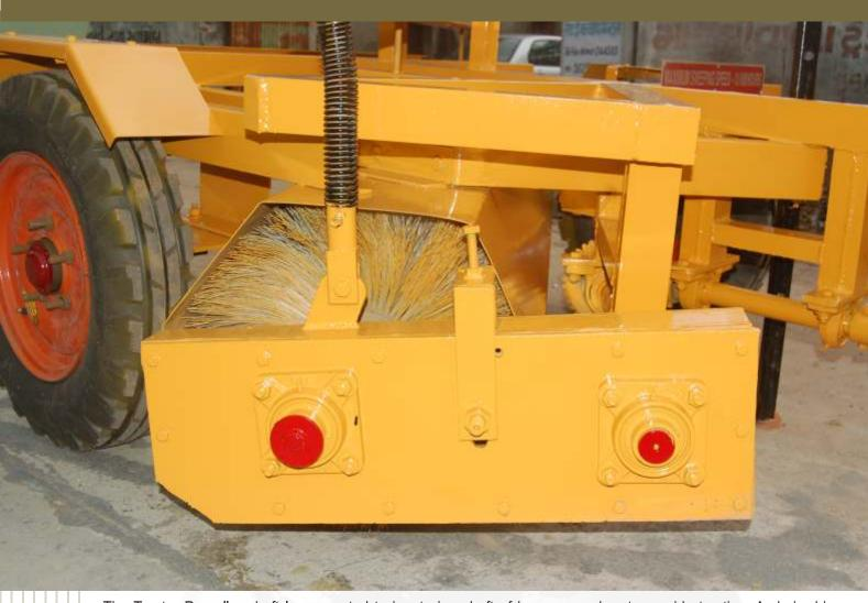
The Tractor Propeller shaft Is connected to input pipe shaft of broom gear box to provide traction. A chain driven mechanism rotates the brush roller.
