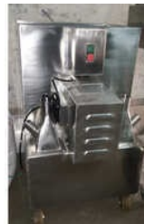
Three Phase Dust Extractor Machine
