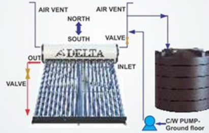
Manual water feeding system
