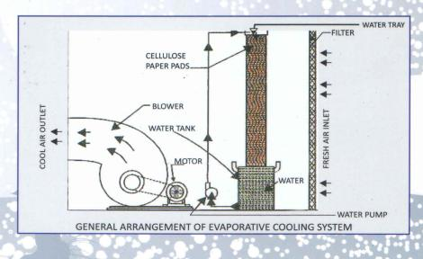
AIRTECH- AIRWAHERS are designed for compactness and rigid construction.
