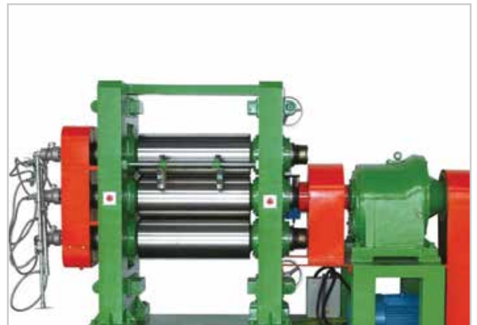
Three roller calendering machine,used for making rubber sheets, and for coating or friction one side or tyre cord with rubber
