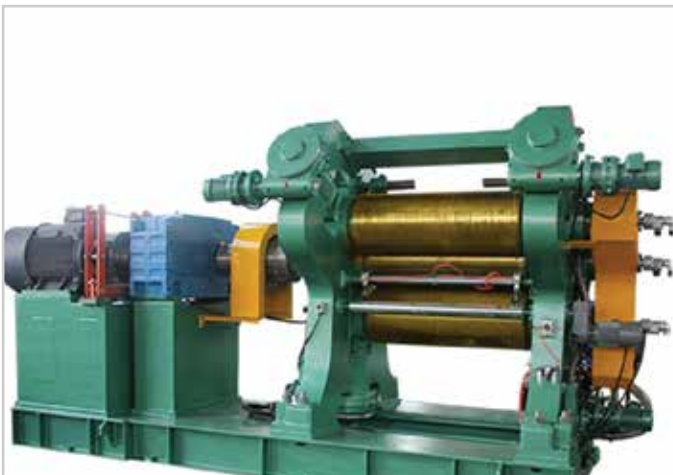
Two roll calender machine,used for making the P.V.C floor tile or automobile tyre, footwear etc
