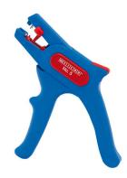
The WEICON Wire Stripper No. 5 has an adjustable length stop from 5 – 12 mm. This allows all flexible and solid conductors of 0.2 – 6.0 mm² (24 – 10 AWG) to be stripped. The length stop can be removed if required. An easy-to-access side cutter is integrated into the tool and can be used up to a cable diameter of 2 mm. It also has exchangeable blades.
