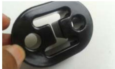
This good quality durable exhaust hanger also called as silencer hanger or muffler hanger used in automobile car parts. we have most of the sizes used in Nissan,Toyota. Volkswagen and we can make as per your size
