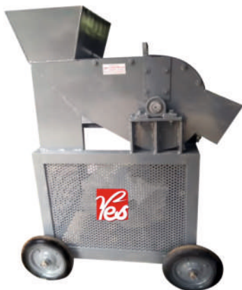
BIO WASTE SHREDDER ( 3/ 5 / 7.5 / 10HP )
