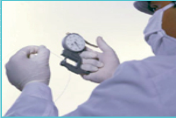
Checking the diameter & uniformity of sutures
