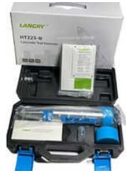
Concrete Testing Hammer
