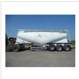
23 Cubic Meter Cement Bulker Tank
