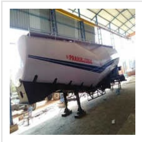
36 Cubic Meter Cement Bulker Tank
