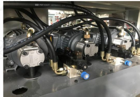
Separate Ele. Motor & Hydraulic Pump for each working station.
