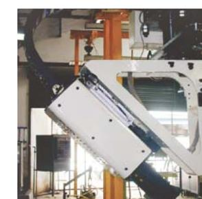
3 Spindle DC Nutrunner for Spark Plug Tightening
