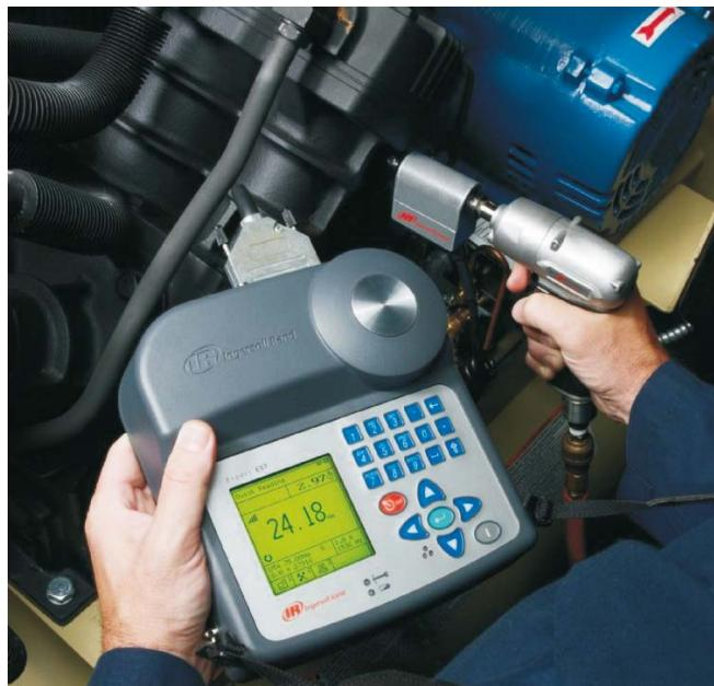
The new Ingersoll Rand EXTA series torque analyser is designed for use with an extensive new range of transducers to measure and record the torque output of all types of fastening tools, including pulse wrenches.
