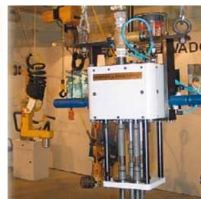
4 Spindle air Nutrunner for Cylinder Head Tightening
