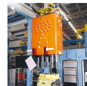
18 Spindle DC Nutrunner for Cylinder Head Tightening
