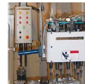
7 Spindle air Nutrunner for Crank Case LH & RH Tightening
