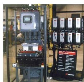
C-Frame Mounted 8 Spindle for Intake Manifold Tightening
