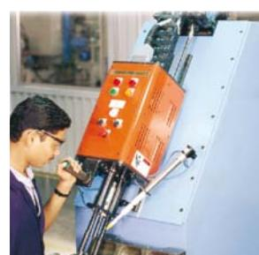
2 Spindle DC Nutrunner for Connecting Rod Tightening
