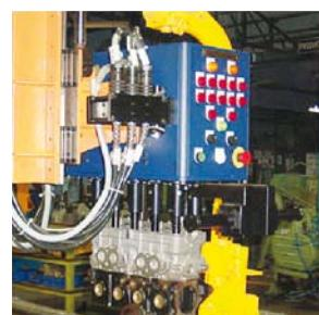
12 Spindle DC Nutrunner for Cylinder Head Tightening
