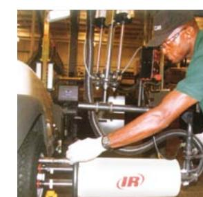
4 Spindle for Wheel Nut Tightening
