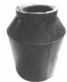
MAY-13 Lift Axle Bush Tata 3118 40mm (ID) × 52mm (OD) × 132mm Height
