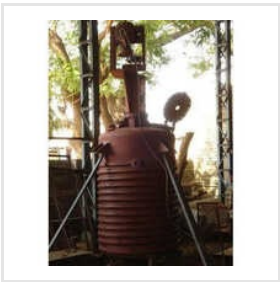
Mild Steel Chemical Reactor
