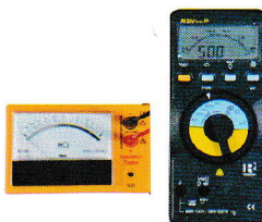
Insulation Tester (Megar) 138
