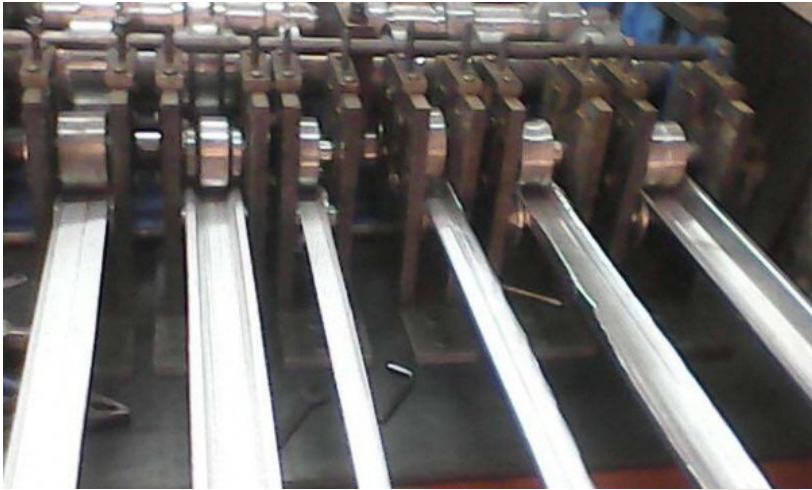
FALSE CEILING ROLL FORMING MACHINE
