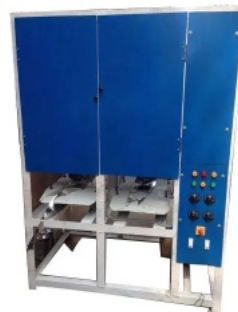
Fully Automatic Dona Making Machine
