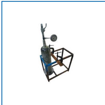
HYDRAULIC ACCUMULATOR PACK
