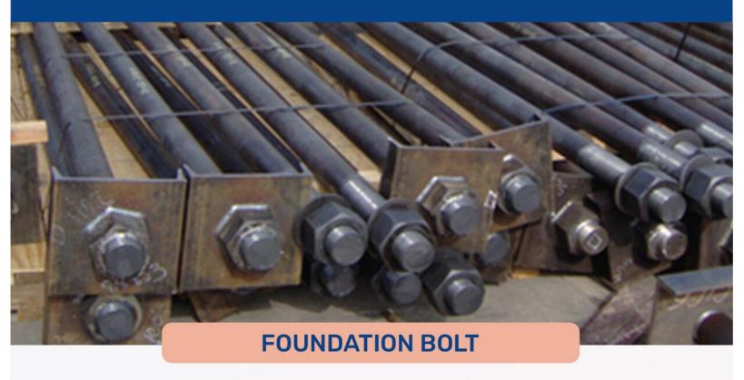
Foundation Bolts are long threaded bolts, straight or bent in different styles, used for anchoring steel profiles and plates to concrete. Foundation bolts are coupled with hex nuts and plate washers to secure the joint. Foundation bolts are often used in bent profile such as J and L.
