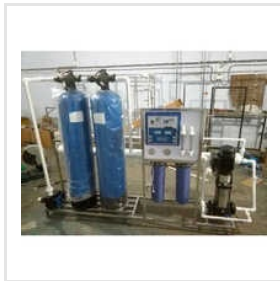
Stainless Steel And FRP And RO Plant
