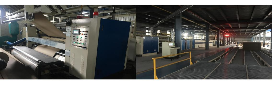
Fully automatic 2500MM corrugator with 150-200mtr running speed.
