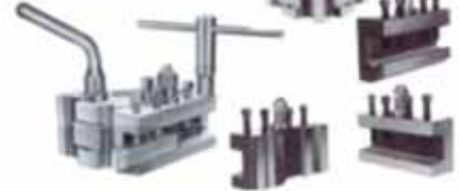
Quick Change Tool Post with multi tool holder
