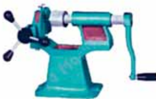
Hand Operated Threading M/c.
