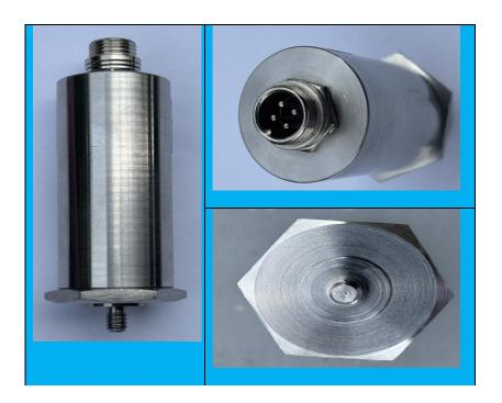
General purpose, top-entry velocity transducer with DC output. Made stainless steel throughout for continuous vibration monitoring in various complicated environments. Internal electronics are enclosed and isolated to minimize noise. Industry standard 4-20mA output proportional to vibration velocity RMS that can connect directly to PLC, DCS and other industrial controllers.
