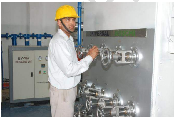
EASY CONTROL VALVES MOUNTED ON THE COLUMN –COLD BOX. Control instrument panel – all pressure flow and temperature readings displayed on one panel.
