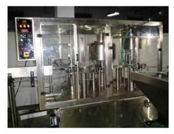
3. The bottles have to be loaded on the mouth of the Infeed Air conveyor. A blower is fitted on top of the frame of the Air conveyor. The air pushes the bottle further automatically and the bottles enter the Monoblock Rinsing, Filling & Capping machine. Total length of Infeed Air Conveyor is 8feet.
