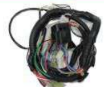
HARNESS WIRING BAJAJ COMPACT
