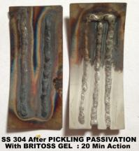
SS 304 Welded Plate SS 304 Argon Weld 20 Min Pickling & **Passivation using** Plate brfore Pickling BTITOSS GEL
