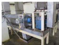
Germ Dewatering Screw Press
