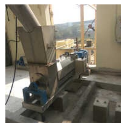
Husk Dewatering Screw Press
