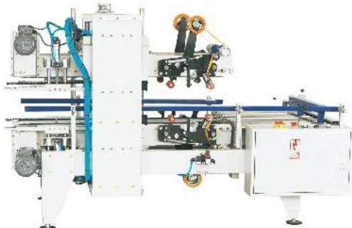
This machine is used to automatically seal carton corners with pressure-sensitive adhesive tape like PVC and BOPP. It is used for the carton in regular shape. Carton sealer can be customized according to customers' requirements so as to meet different customers' needs. The machine has been widely used in the food industry, chemical fiber, tobacco redrying, pharmacy, publish, air conditioning, household appliance, ceramics, hot work and so on.
