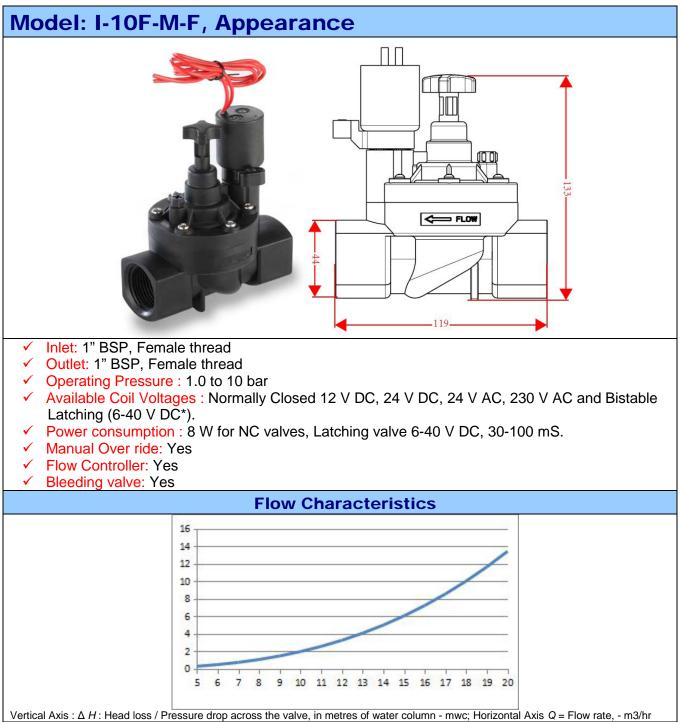
\* Latching coil pulse width and voltage depends and varies on operating conditions
