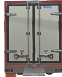
Door Frame : Door frame "C" Profile having 2mm SS Sheet.
