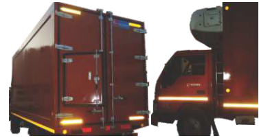
Radium Line : Front side & back side yellow reflection radium line for night time.
