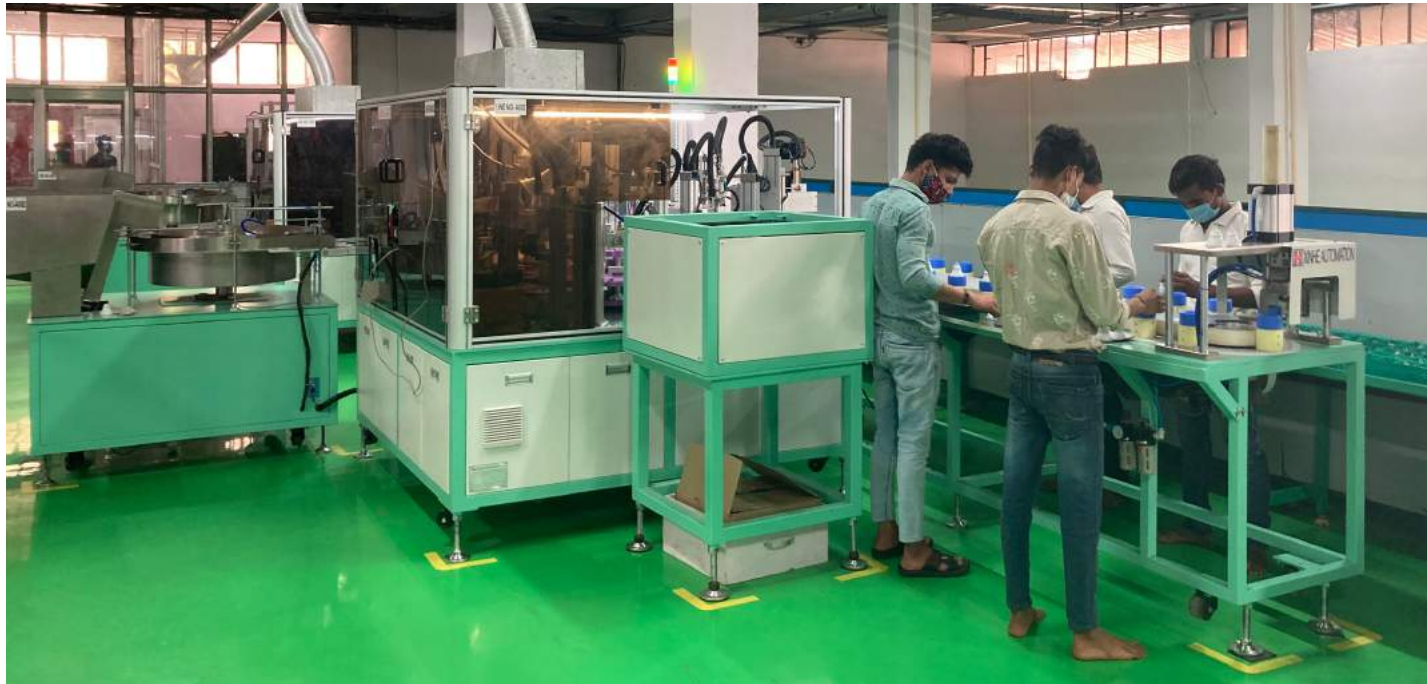
Fully Automatic LED Bulb Assembly Plant with a capacity of 1 million/ month
