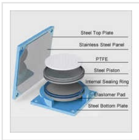
Pot Bearing Components
