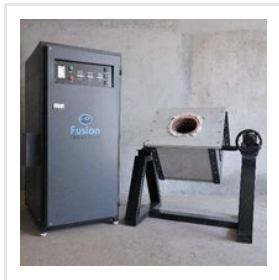
Induction Melting Furnace
