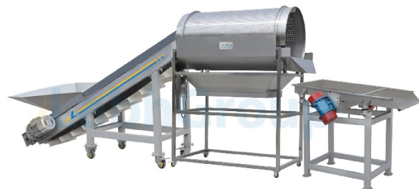
Cooling & Separating Drum
