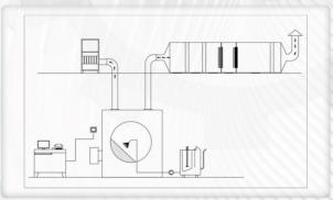
Tablets Pellets are allowed for roll (smooth rolling) while a coating medium is sprayed with atomization using - engineered spray nozzle and a positive displacement Pump. Hot air properly filtered with setable temperature and humidity, is bubbled through rolling bed of Tablets/Pellets evaporating the liquid and ensuring even and smooth coat of solids from spray solution. A proper heat and mass balance is necessary for coating quality with energy conservation
