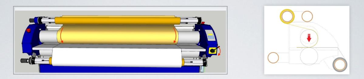
Then press the middle of media by hand while twist the valve handle in clockwise direction, to fall down the up-roller, which will fix the media and the film, ensure there is no any relative movement between them.
