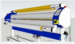
Put on the media for the media loading rod, also put on paper tube for the back paper collecting rod.
