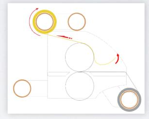
Frap the film back to the film loading rod until the film cling to the roller tightly.
