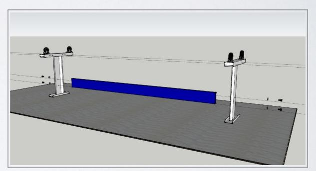
2. Assembly the color blue beam first, please add gasket for the screw. Attention: don't tighten the screw right now.
