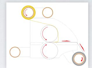
Confirm the roller has laminated the film onto the end of media and still not lost pressing it, then loose the feet pedal to stop the rotation of the roller.
