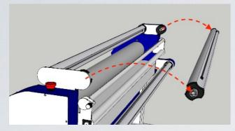
Open the bracket shell, pull out the film loading rod from the bracket slot.
