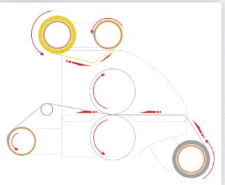
If the machine equipped the back cutting device, the laminated media should cover the lower supporting rod of the cutting device. Just like the picture showed:
