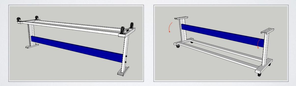
4. Then tighten the screws. The assembly of connections beams finished.
