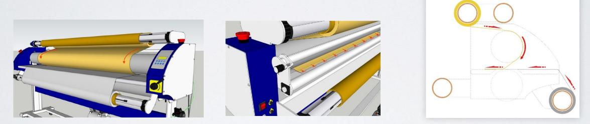
Pull the end of the film roll down, through the bottom of up-roller, make sure the end of film roll align to the end of the media.
