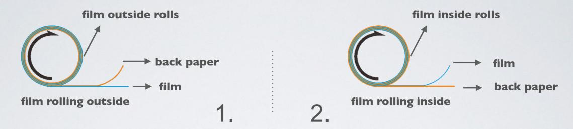
Accordingly, there should be two film installing methods as below, please be more attention on the running direction:
