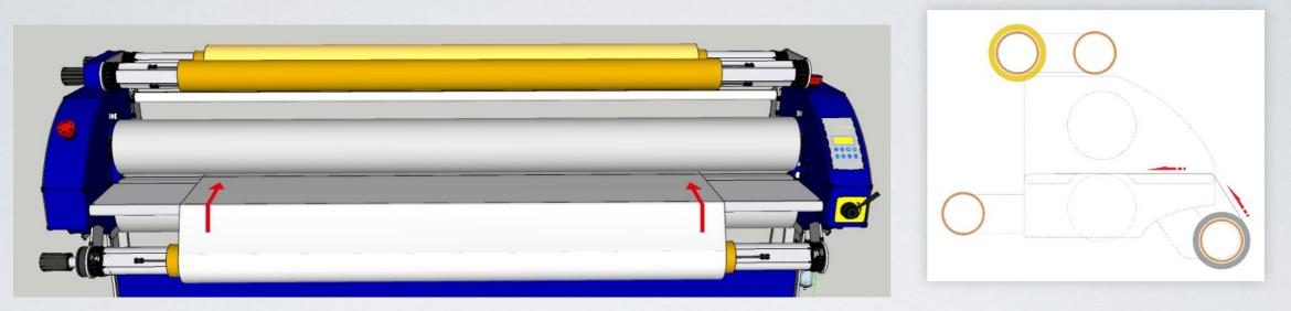
Pull the end of media up to the front platform, then flatten it, ensure the media end cover and over the rollers around 15cm.
