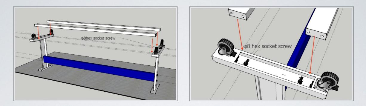
3. Assembly the 2 units of white beam. Because the small space inside the machine legs bottom slot, better correct screws with bare hand, it's more convenient and effectual.
