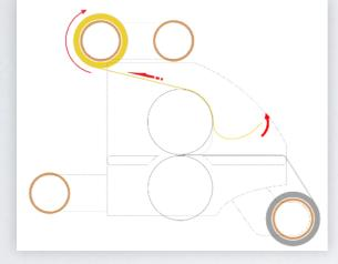
Then unfold the end of yellow back paper and pull it up to the back paper collecting rod meanwhile rotate the film loading rod in backward to frap the film.
