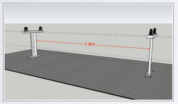
Put the legs upside down on the ground, better pave a soft materials under the bottom to protect the painting. The distance between the them should be around 1.8m.
