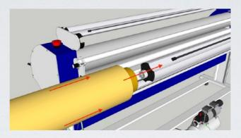
Plug the film roll onto the film loading rod, please be more attention on the rolling direction(reference on the diagram in last page).
