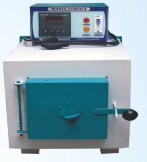
**HEATING ELEMENTS AND TEMPERATURE CONTROLLER:** Silicon carbide heating elements are fitted to achieve the temperature upto 1400°C. The temperature is controlled by FUJI/ HONEYWELL / MEXTHERM PID Microprocessor based Digital Temperature Indicator cum controller with temperature stability of  $\pm$  1 °C. The controller with 8 programmes and 4 step in each segment with ramp and soak to display the set temperature with dwell auto cut off at set point.
