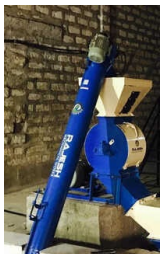
Grinding Machine & Conveyor
