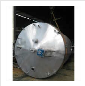
Mild Steel Storage Silo Tank
