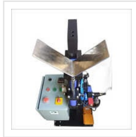
Hydro Pneumatic Corner Crimping
